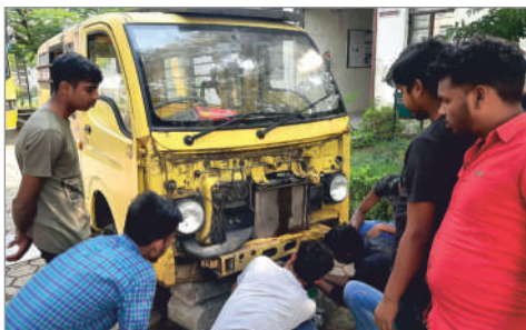
Conversion of old Tata Magic in to electrical vehicle by CRE-RNTU Bhopal
